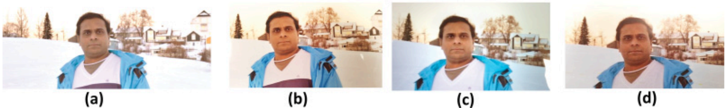
Fig. 3. Illustration of face artifacts generated using the legitimate user photo obtained from a social website: (a) photo from the social website, (b) inkjet print, (c) electronic display, and (d) laser print.
