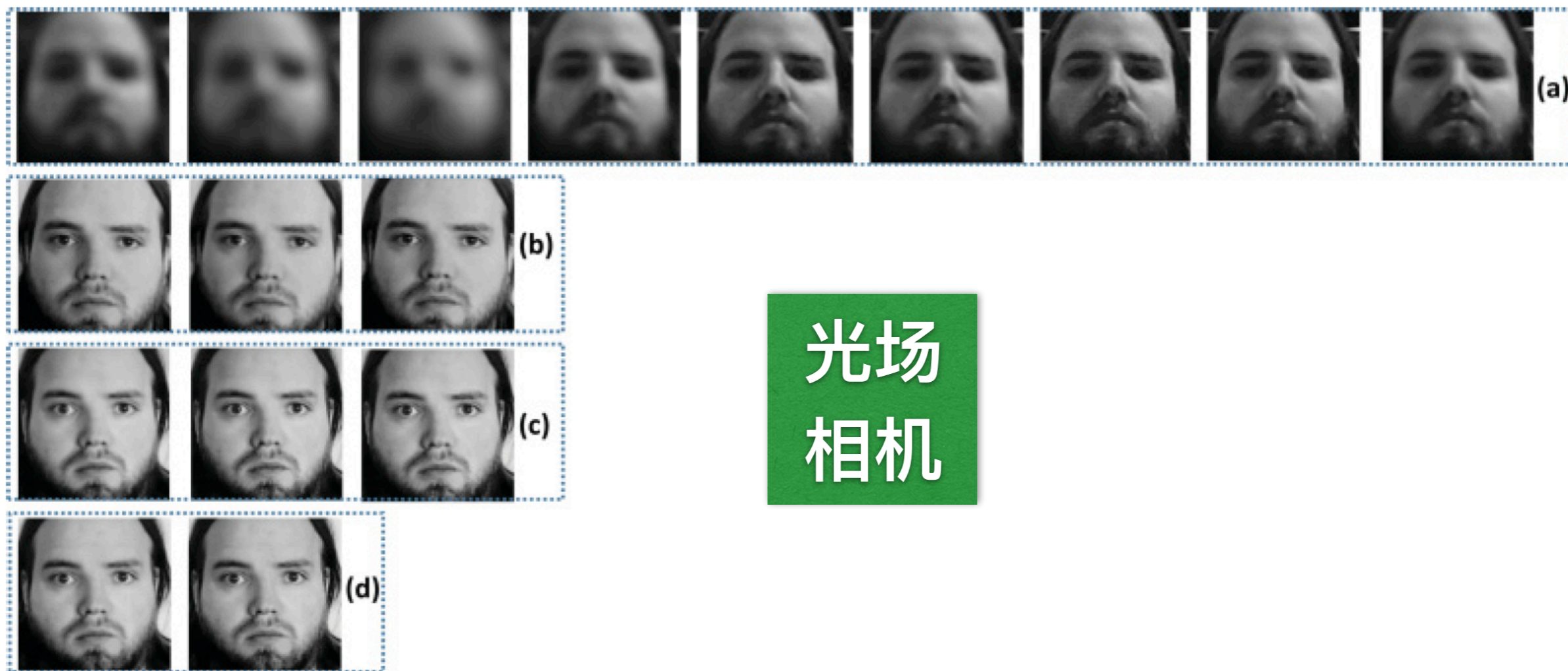
Fig. 7. Illustration of using a variation of focus rendered by the LFC to detect face artifacts: (a) real face focus images rendered by the LFC; (b) inkjet print attack focus images rendered by the LFC; (c) display attack using iPad focus images rendered by the LFC; and (d) laser print attack focus images rendered by the LFC
