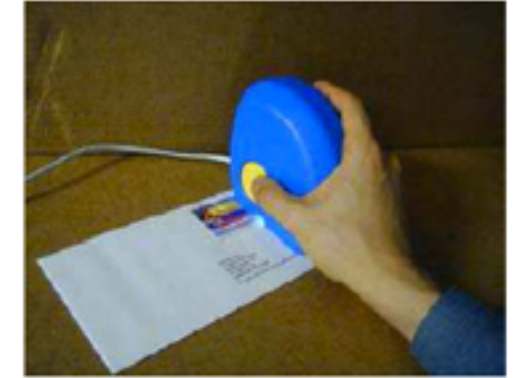
Figure 3: a) The Fiberfingerprint method; b) Verification device used to extract the substrate individualities (Source: Metois et al. (2002))
